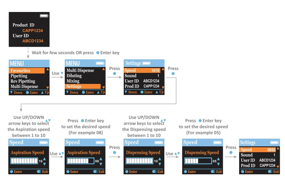
Exit: Press of for 2 to 3 seconds to come out from the existing mode
