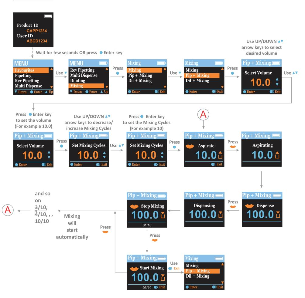
Exit: Press of for 2 to 3 seconds to come out from the existing mode
