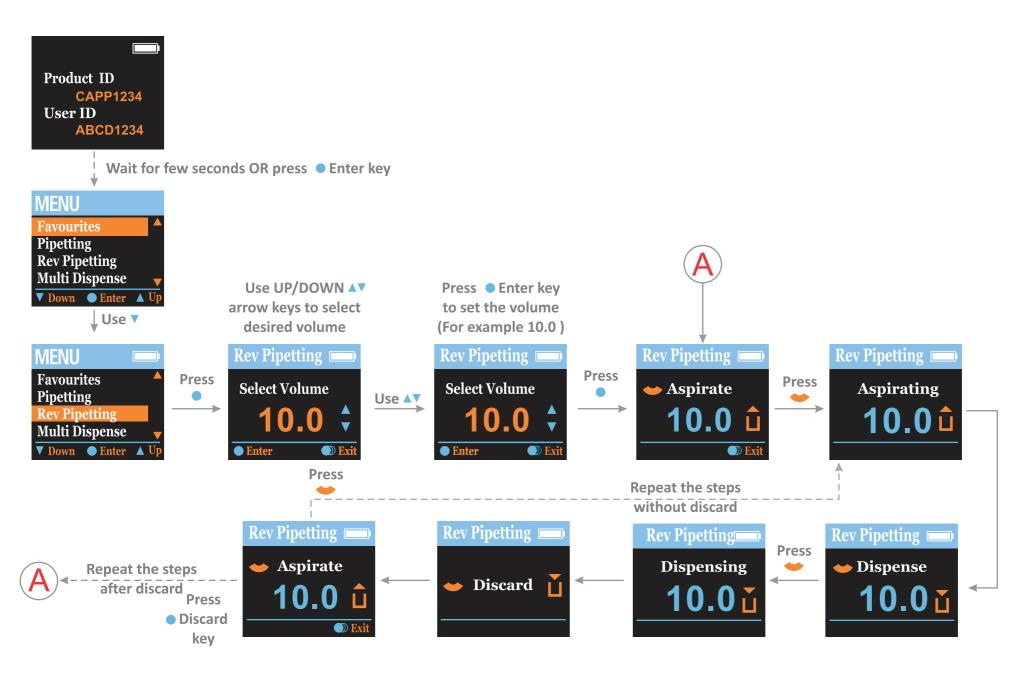
Exit: Press of for 2 to 3 seconds to come out from the existing mode
