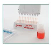
Transfer 100 µL Red Stop from reagent boat to antibody wells.
