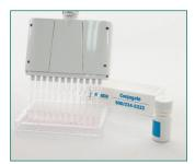
6. Transfer 100 µL conjugate from reagent boat to antibody wells using 12-channel pipettor. Incubate for 10 minutes.
