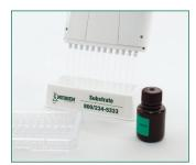
Transfer 100 µL substrate from reagent boat to antibody wells using 12-channel pipettor. Incubate for 10 minutes.
