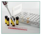
1. Add 150 µL controls and extracted samples to transfer wells.
