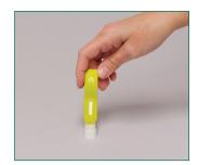
Dip the Reveal 3-D device into the liquid in the lid, ensure that the cavity is saturated with the liquid.
