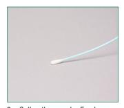
Gather the sample. For dry surfaces moisten with extraction solution. Do not premoisten for wet surfaces.
