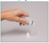
Open Type 7 extraction buffer sachet and add to a sample tube.
