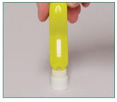
Leave the cavity saturated until the liquid is seen running into the test window.
