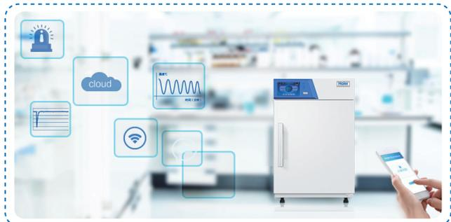
Through the mobile app, the status of the incubator can be checked in real time, and information such as temperature alarm, sensor error alarm and door ajar can be controlled with one button, which provides more security for the experiment process.
