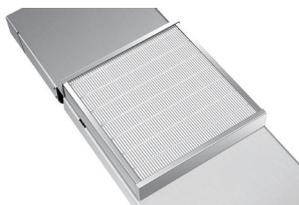
The optional HEPA high-efficiency filtration system combined with the unique air duct circulation design can continuously filter pollutants (biological pollutants and suspended particles) in the cabinet, ensuring that the incubator can reach the ISO class 5 clean room within 5 minutes after the external door is closed, which is equivalent to the class 100 environment of the 209 E standard of the united states
