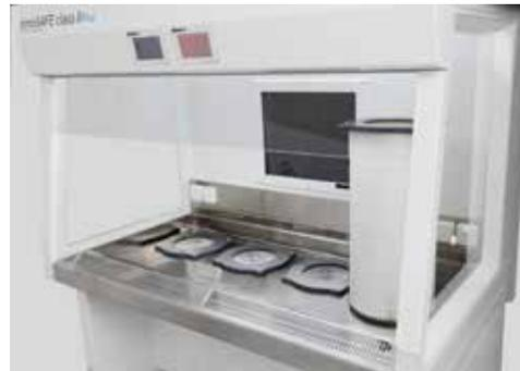
**Optional H14 pre filters according to DIN12980**
