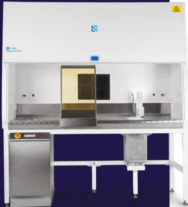
n-Safe Isotope cabinets are available with a lead shielding of 1-50 mm Pb, depending on the customer's requirements. The cabinets' bottom, sides and back wall can be covered with 1-50 mm lead plates, which are encapsulated in stainless steel. n-Safe Isotope cabinets also feature a slidable front on ball bearings made of 1-50 mm Pb-equivalent lead glass.
