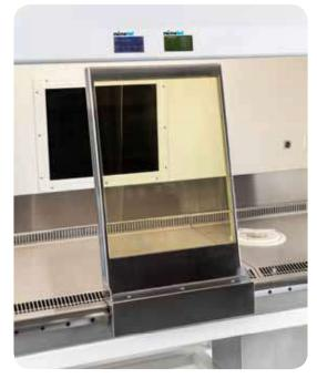
Slidable radiation shield with 1-50 mm Pb equivalent lead glass
