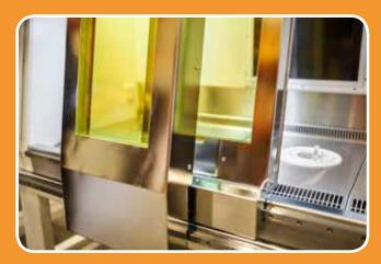
Radiation shielded slidable fronts for best possible ergonomics. Split in 30 plus 20 mm Pbequavilent lead glass which can be used separately or together for 50 mm Pb-equavilent.
