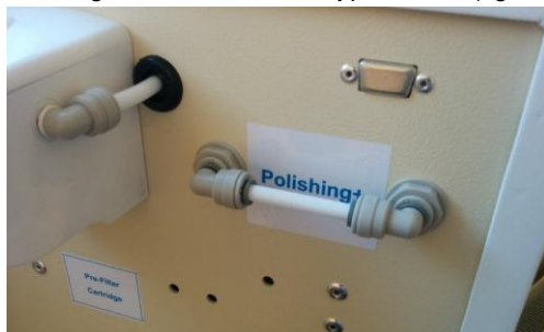
Figure 33. Inserted bypass tube.
