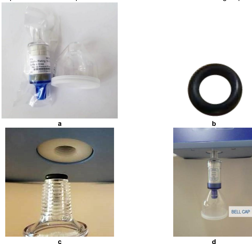
Figure 20. 0.22 \mu m filter dispenser installation.
