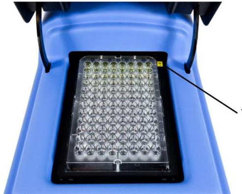
**Figure 3. Correct microplate placement.**
